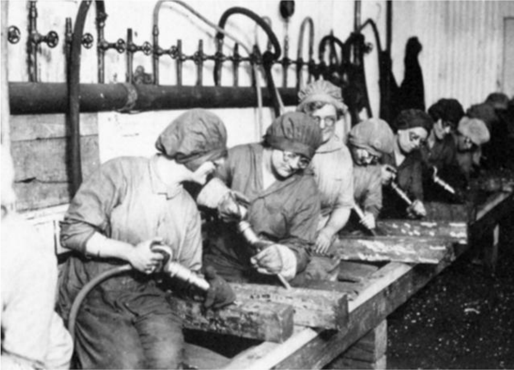
Women workers in ordnance shops (military supply shop), Midval Steel and Ordnance Co., Nicetown, Pa. Hand chipping with pneumatic hammers.
